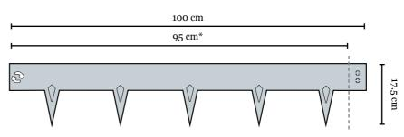
\*working length. To calculate how many segments you need for the total required length you have to edge, divide this length by 0.95.
