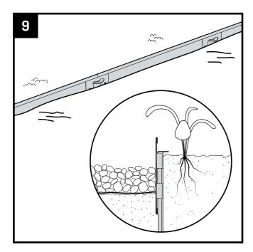
Backfill the channel with soil, sand or another material. Then lay grass, gravel or another type of ground cover up to the edging.
