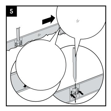
Widen the channel dug at the ends of the profiles if necessary. Push the connector strips under the top and bottom edge of the profile. Press the connector strips against the profile and push the fixing stake through the openings in the connector strips. Leave half of the fixing stake protruding above the profile.
