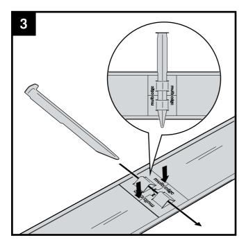
Press the connector strips against the profile. Push the fixing stake through the openings in the connector strips and leave half of the fixing stake protruding above the profile.
