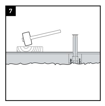
Gently tap down the profiles to the desired height. Use a wooden block to avoid damaging the profiles. For stability, leave no more than 10 cm of the profile protruding above the surface of the soil.
