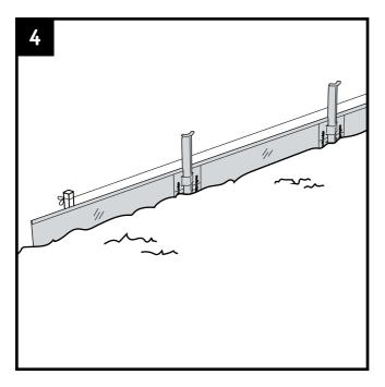
Place the profile loosely in the channel dug. Bend the profile by hand to create a curved contour. Bend the profile around a solid object (e.g. the edge of a workbench) to create an angle. Or use the optional corner pieces (step 6). Cut off any excess length using a grinder or metal saw.
