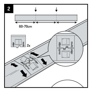
Before the profiles are installed in the soil, fit 2 connector strips at 60-70 cm intervals for attaching the fixing stakes to the profile. Do this by pushing a connector strips underneath the top and bottom edge of the profile. Make sure that the connector strips fit together.
