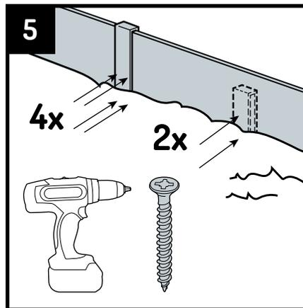
5 Gently tap down the edging to the desired height using a rubber mallet. Screw the fixing stakes to the edging using 2 stainless steel 4 x 30 mm screws. Screw down any fixing stake that has been used as a transition between two profiles using 4 screws.
