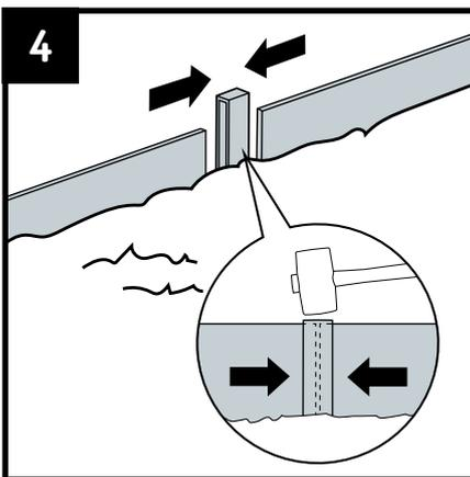
4 It is possible to insert the ends of the edgings into a fixing stake profile. This is not necessary but creates a stable, smooth transition. Smooth corners can be created by sawing through the edging and placing them against each other at the desired angle.
