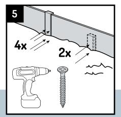
Gently tap down the edging to the desired height using a rubber mallet. Screw the fixing stakes to the edging using 2 stainless steel 4 x 30 mm screws. Screw down any fixing stake that has been used as a transition between two profiles using 4 screws.
