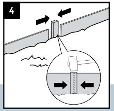
It is possible to insert the ends of the edgings into a fixing stake profile. This is not necessary but creates a stable, smooth transition. Smooth corners can be created by sawing through the edging and placing them against each other at the desired angle.
