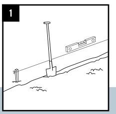
Dig a channel. Make sure that at least half of the edging is able to disappear into the channel. For straight edging, mark out the line along which the Multi-Edge ECO is to be installed using twine and pegs.
