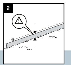
Place the edging into the channel. Make sure that at least half of the edging is in the ground. The edging is even more stable when it is inserted deeper into the ground. Cut off any excess length of edging using a hand saw for wood.
