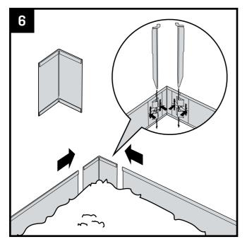
For extra neat 90° angles, use the optional corner pieces. Connect the corner pieces to the profiles using the connector strips. Press the connector strips against the profile and push the fixing stake through the openings in the connector strips, leaving half of the fixing stake protruding above the edging profile.
