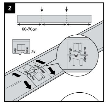
Before the profiles are installed in the soil, fit 2 connector strips at 60-70 cm intervals for attaching the fixing stakes to the profile. Do this by pushing a connector strips underneath the top and bottom edge of the profile. Make sure that the connector strips fit together.
