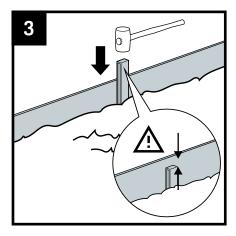
Place fixing stakes at 50 cm intervals along the edging. Tap these into the ground using a rubber mallet. Make sure that the fixing stakes protrude a few cm lower than the top edge of the edging. Once installed, the fixing stakes will no longer be visible.
