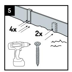
Gently tap down the edging to the desired height using a rubber mallet. Screw the fixing stakes to the edging using 2 stainless steel 4 x 30 mm screws. Screw down any fixing stake that has been used as a transition between two profiles using 4 screws.
