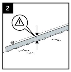
Place the edging into the channel. Make sure that at least half of the edging is in the ground. The edging is even more stable when it is inserted deeper into the ground. Cut off any excess length of edging using a hand saw for wood.
