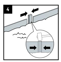
It is possible to insert the ends of the edgings into a fixing stake profile. This is not necessary but creates a stable, smooth transition. Smooth corners can be created by sawing through the edging and placing them against each other at the desired angle.
