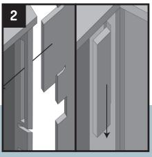
Insert the hooks of one panel into the slots of the other and slide down to connect.
