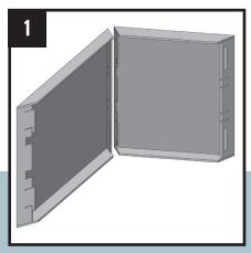
Each panel has two different sides. One side has two hooks and notches, the other has two slots and clips. Place panels with one of their sides facing each other.
