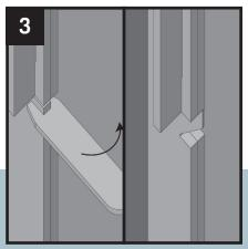
To ensure the panels don't come loose when moved, use the provided bending tool to bend the clips over the notches.
